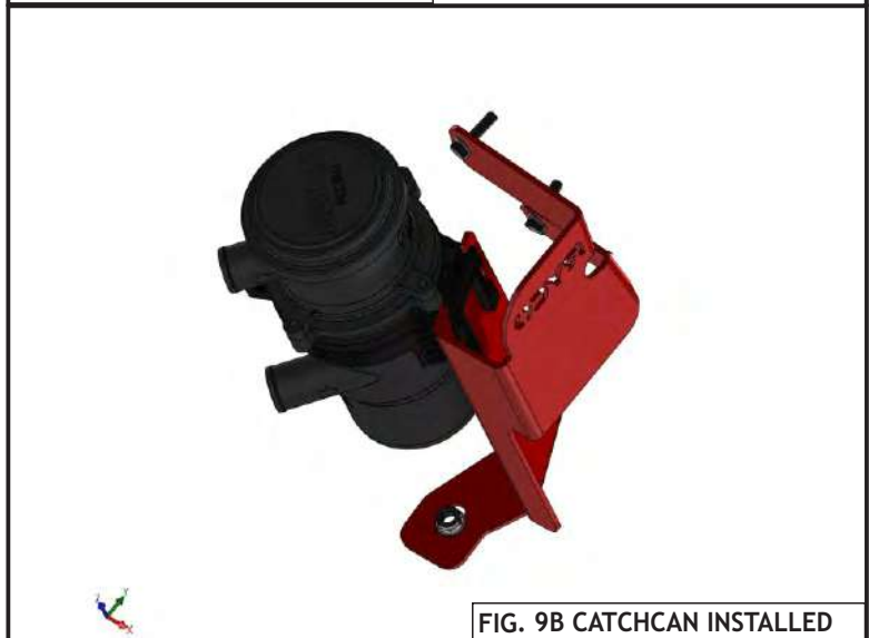
FIG. 9A CATCHCAN INSTALLATION
