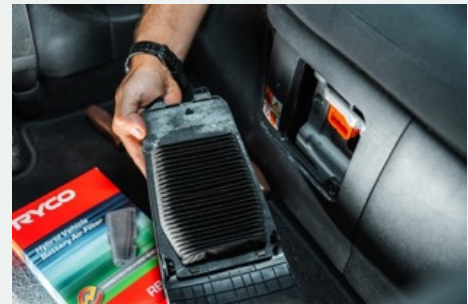
STEP 5A Once flap is released, remove old battery filter by releasing the filter from the tabs holding it in place by pulling away from OEM housing flap. Then install new battery air filter in same orientation as old filter was installed.
