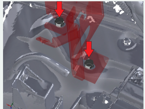
FIGURE 4C FB9810FC BRACKET INSTALLATION
